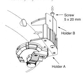
3. Tighten holders "A" and "B" using the screw (5 x 20 mm).
