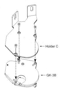
3. Secure Holder "C," with the controller attached to it, to Holder "B" using the flat washers, spring washers and screw (5 mm x 8 mm).
