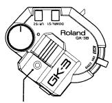
Put the flat-head screw (3x16 mm) through this hole.
