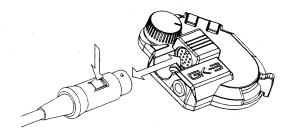
Before playing, be sure to wrap the cable around the guitar strap near the end pin. This will prevent the excess strain on the cable that can end up damaging the bass or the GK-3B.
