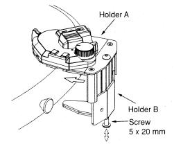
3. Tighten holders "A" and "B" using the screw (5 x 20 mm).
