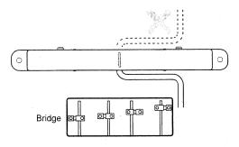
\* Install the divided pickup close to the bridge: In any case, do not install the pickup more than 50 mm away from the bridge.
