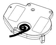
4. Secure the controller with the supplied flat-head screw (3 x 16 mm).
